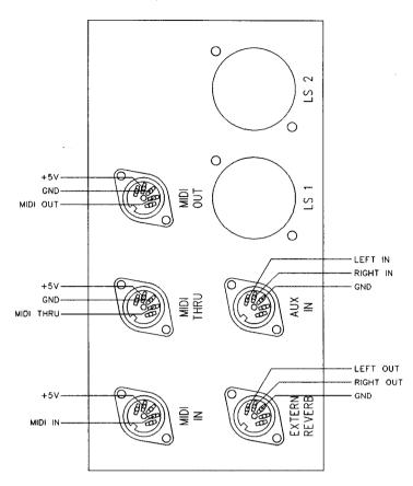
At the rear of the console (seen from the rearside at the very right, in the middle) several DIN connectors are located (see above drawing). The functions of these connectors are the following:
